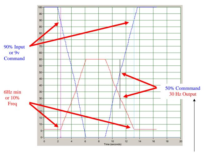
Also, if the command signal becomes 5v or 50%, the drive would be running at 30Hz.
