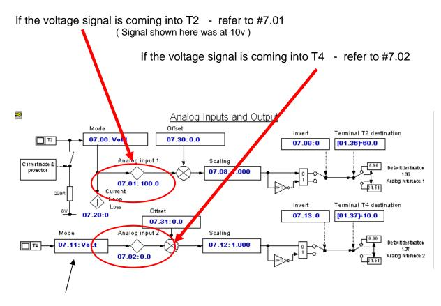
If T4 is selected as the command input, the mode #7.11 must be changed to Volt.
