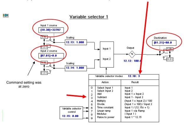
I elected to set Input 1 Source to a free drive register in menu 18. I chose #18.30 and set it to a value of 32767 which is the maximum range of that register. The Variable Selector will treat that value as 100%.
